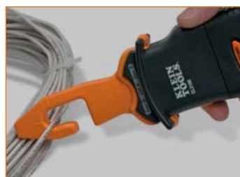
Separate Tie-Wrapped Wires
